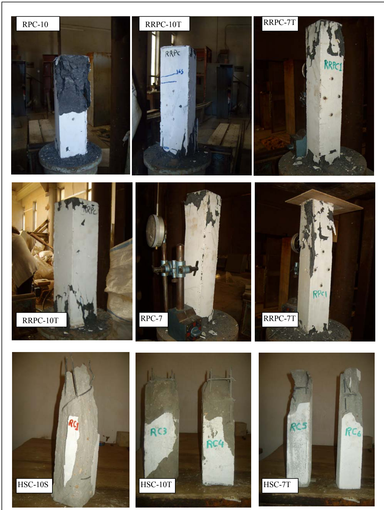
Fig.(3) Failure Mode of Column Specimens
