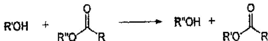
Fig. (1): illustrated Transesterification: alcohol + ester ® different alcohol + different ester
