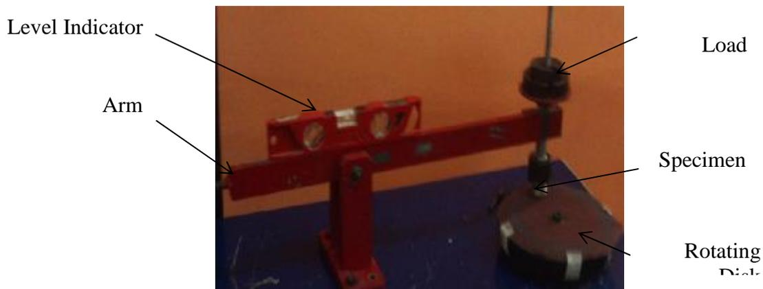
**Fig (2) Apparatuses of adhesive wear test**
