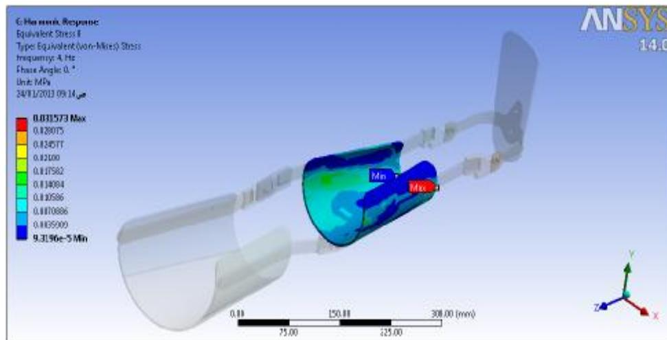
**Fig.(20): The Von-Misses stress due to harmonic body motion (acceleration) at calf shank contact with gastrocnemius muscle for KAFO**
