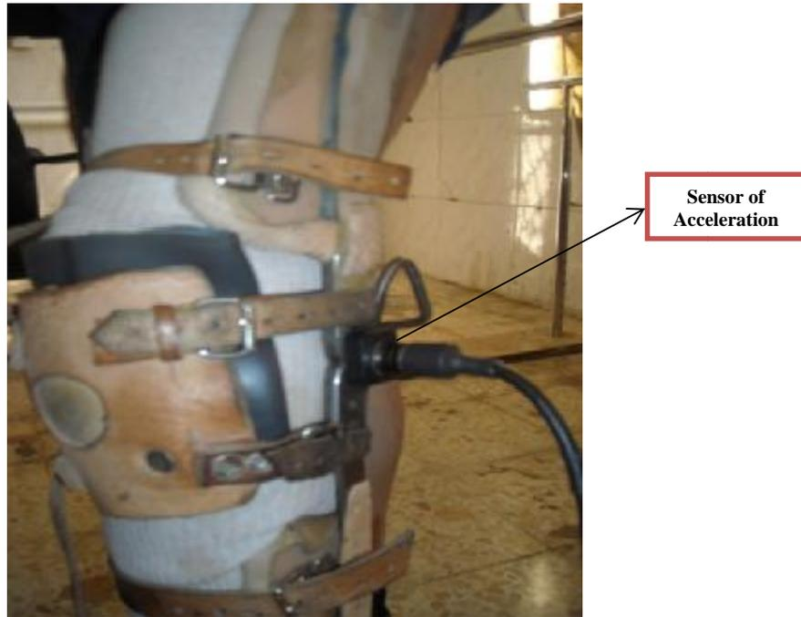
**Fig.(1) : Acceleration sensor device.**
