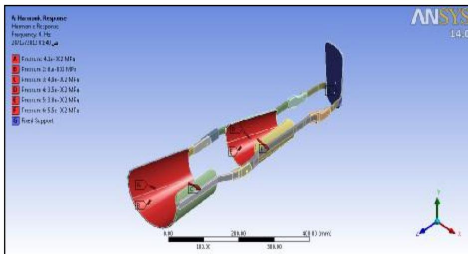
Fig.(4): The model subjected to maximum pressure load
