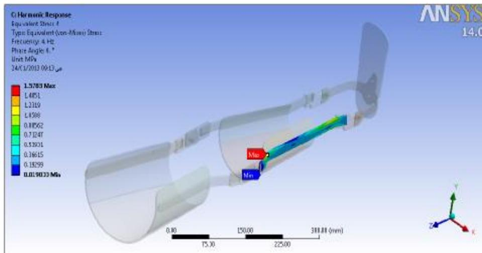
Fig.(14): The Von-Misses stress due to harmonic body motion (acceleration) at bar contact with soleus muscle.
