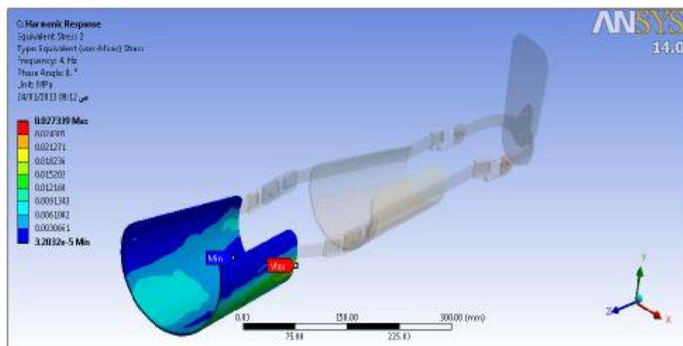
Fig.( 18): The Von-Misses stress due to harmonic body motion (acceleration) at thigh calf contact with semitendinosus for KAFO
