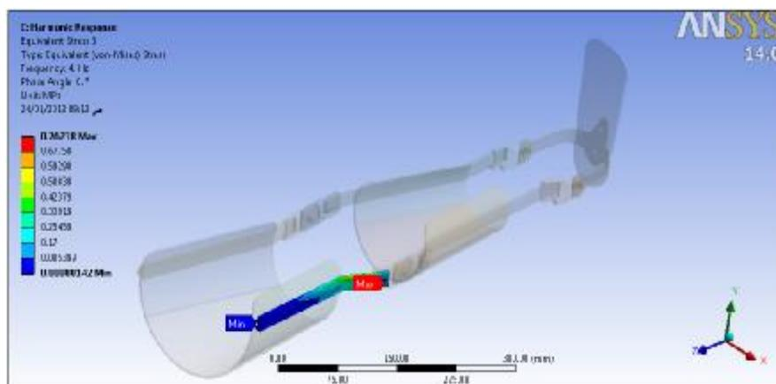
**Fig.(10) : The Von-Misses stress due to harmonic body motion (acceleration) at bar contact with Gracilis muscle.**
