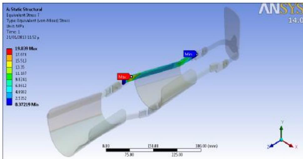
Fig.( 15): The Von-Misses stress due to loading boundary condition (IP) at bar contact with peroneus longus muscle
