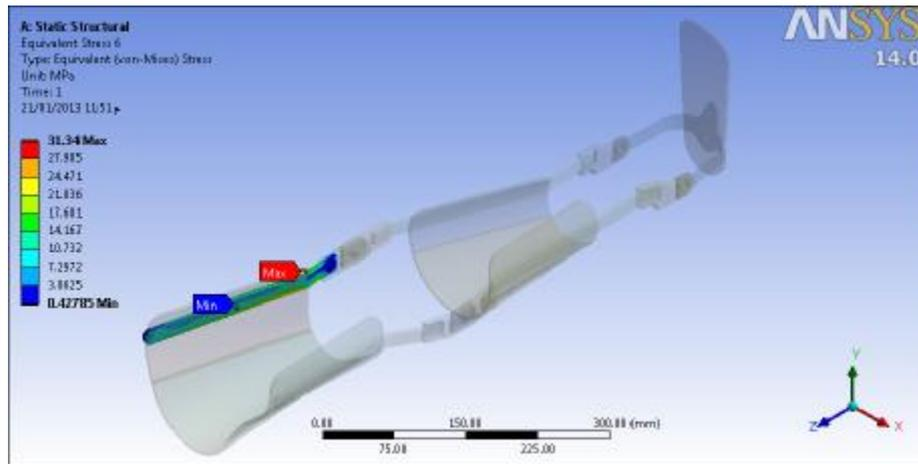
Fig.(11) : The Von-Misses stress due to loading boundary condition at bar contact with vastuslateralis muscle
