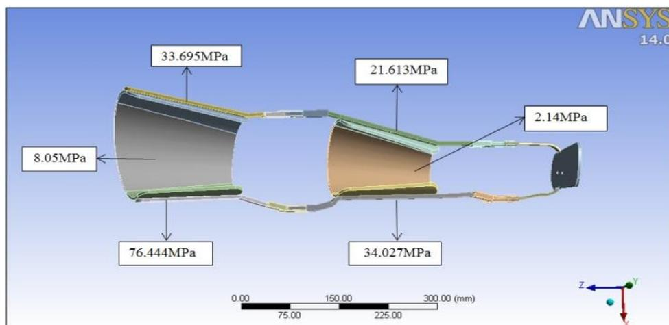
**Fig.(21): Total stress result from applied pressure and acceleration on the model**
