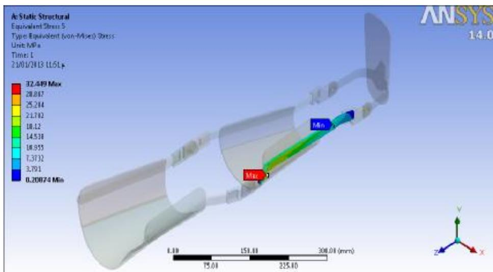
Fig.(13): The Von-Misses stress due to loading boundary condition (IP) at bar contact with soleus muscle.
