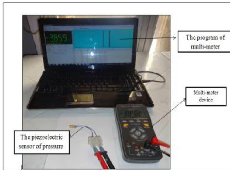
Fig. (3) : the multi-meter and piezoelectric are interface with the computer
