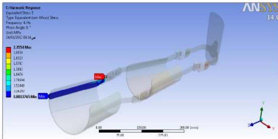
Fig.(12) The Von-Misses stress due to harmonic body motion (acceleration) at bar contact with vastuslateralis muscle.
