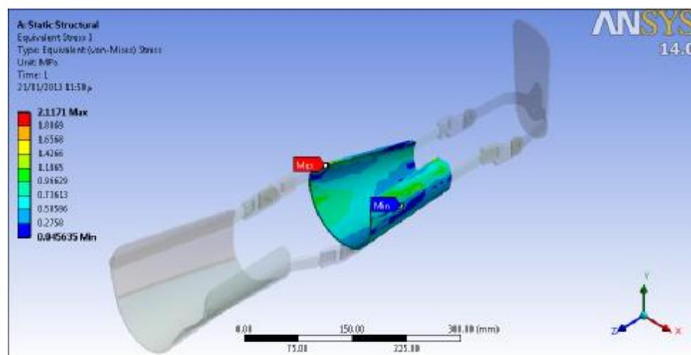
Fig.(19):The Von-Misses stress due to loading boundary condition (IP) at calf shank contact with gastrocnemius muscle for KAFO
