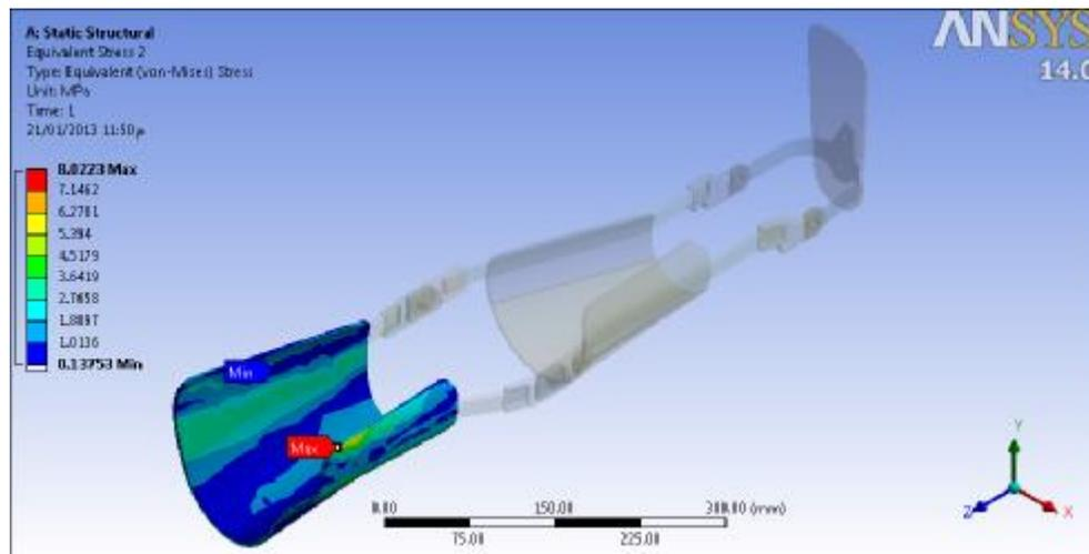
Fig. (17) : The Von-Misses stress due to loading boundary condition (IP) at thigh calf thigh contact with semitendinosus for KAFO
