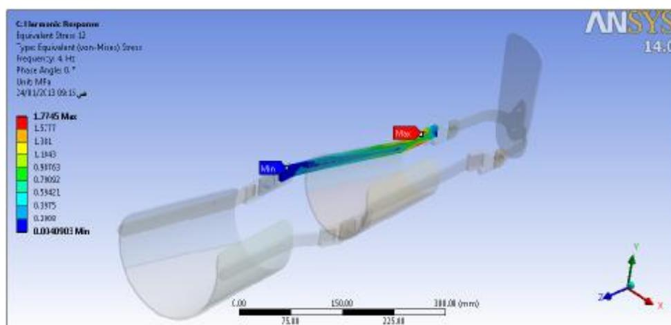
Fig.(16): The Von-Misses stress due to harmonic body motion (acceleration) at bar contact with peroneus longus muscle
