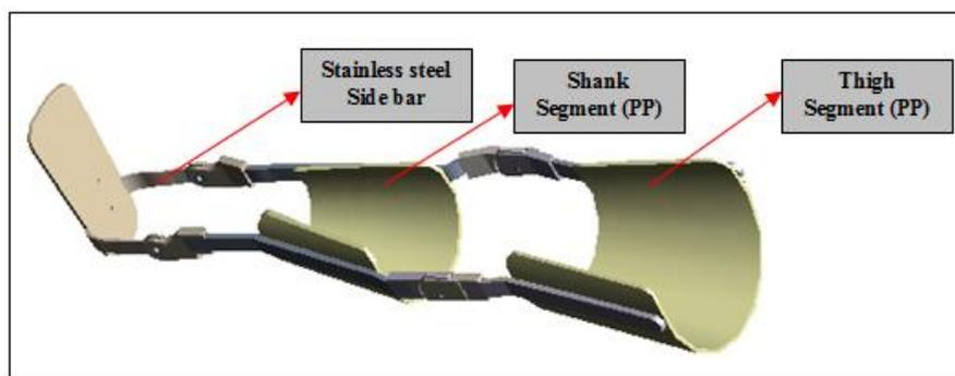
**Fig.(6) : Graphing of the geometry and material selection in KAFO's**
