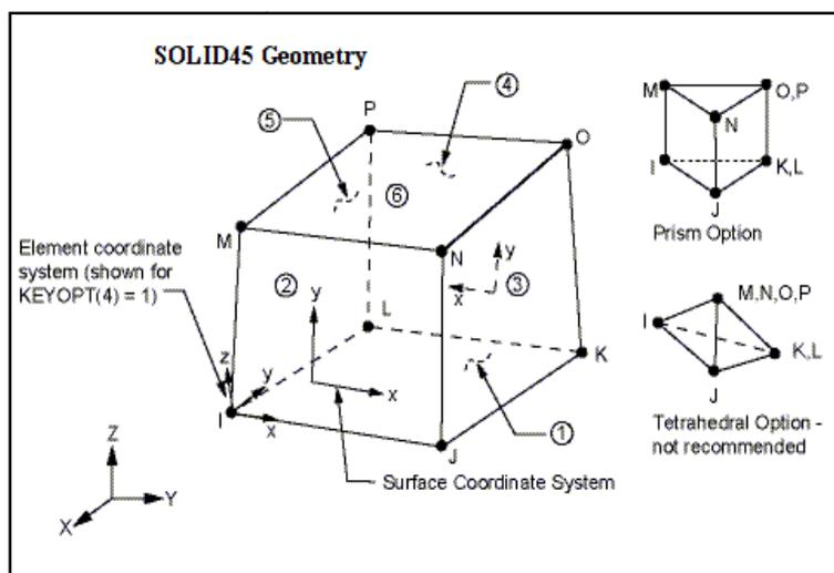
**Fig.(8): Solid 45 element geometry**
