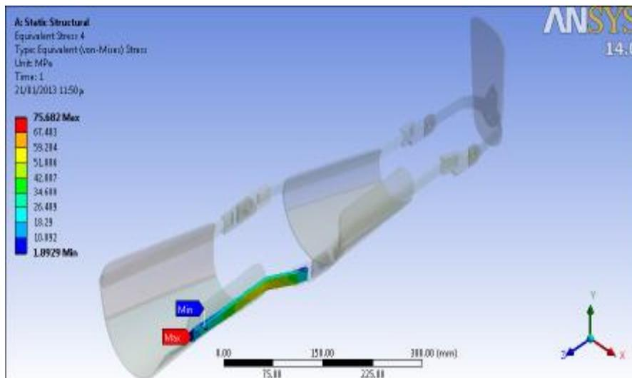
**Fig.( 9) : The Von-Misses stress due to loading boundary condition (IP) at bar contact with Gracilis muscle.**
