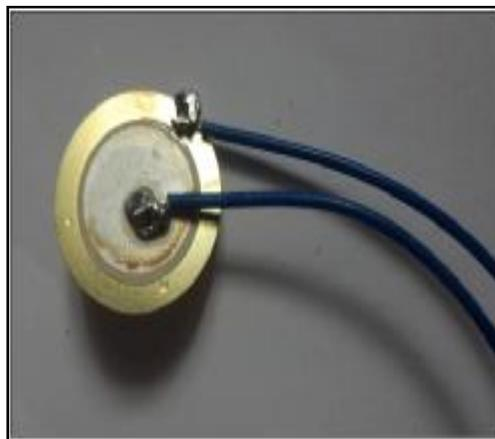
**Fig.(2): The piezoelectric sensor**
