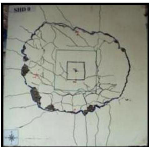
Plate (x) Tension Face for Slab SHD.
