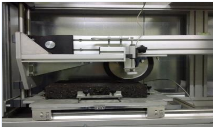
Plate (2) Sample Hold under Wheel and LVDT Transducer to Monitoring Rut Depth
