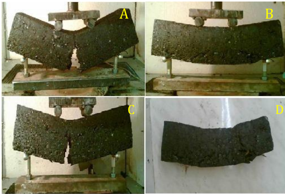
Plate (3) Failures of Beams Samples: A-Unreinforced Sample, B-Bottom Embedded Reinforcement, C- Middle Reinforced Samples, D-Doubly Reinforcement
