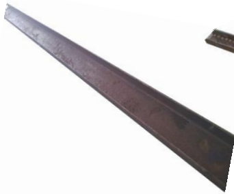
Plate 1: Steel channel devoid of studs for TB-NS
