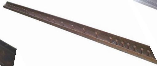
Plate 2: Steel channel and studs for TB-NU D/R
