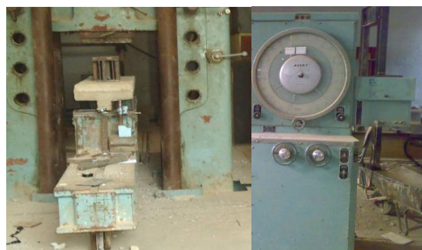
Plate 0: The universal testing machine (2000) M.F.L.system) with a typical test beam
